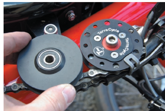
BELOW: fitting a replacement idler to a Challenge trike.
