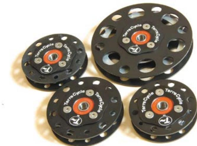
(usually) linked issues of noise and efficiency. With plain plastic pulleys, the chain runs on the tops of the links, and these aren't flat at all, typically with a bump over each chain pin. So the chain tends to drop slightly between the bumps, then rise again, as the chain passes over the pulley. This all causes vibration, noise, and that takes energy which is lost as 'inefficiency'.
