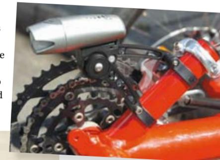
support a short section of 1" tubing onto which you can fit any manner of accessories. An optional 'tab' also provides a bolt location for dynamo lights, for example. The two legs can be set at any angle, and come in 50, 75 and 100 mm lengths. It's all held together with stainless steel hardware.
